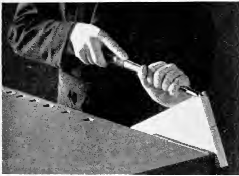
Fig. 8. Chiseling with the Grain.
